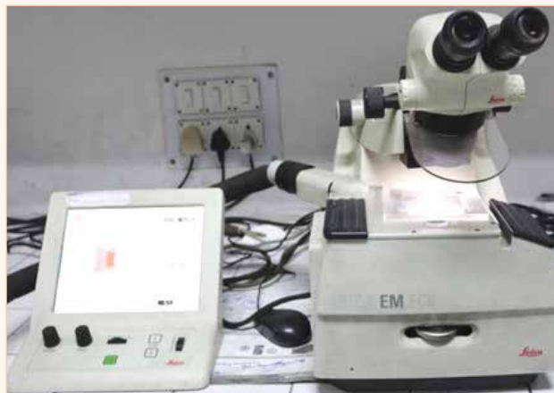
Figure 6 : Ultramicrotome (Leica UC-6)
